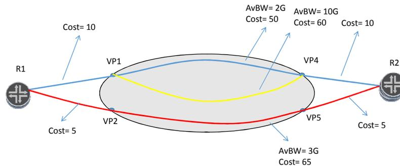
Figure 6 - IP+Optical Path Computation Example with multiple choices
